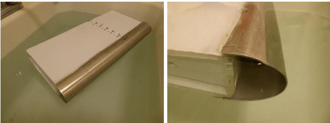
**Figure 3 Flaperon Model #2 floating with void full of water**
